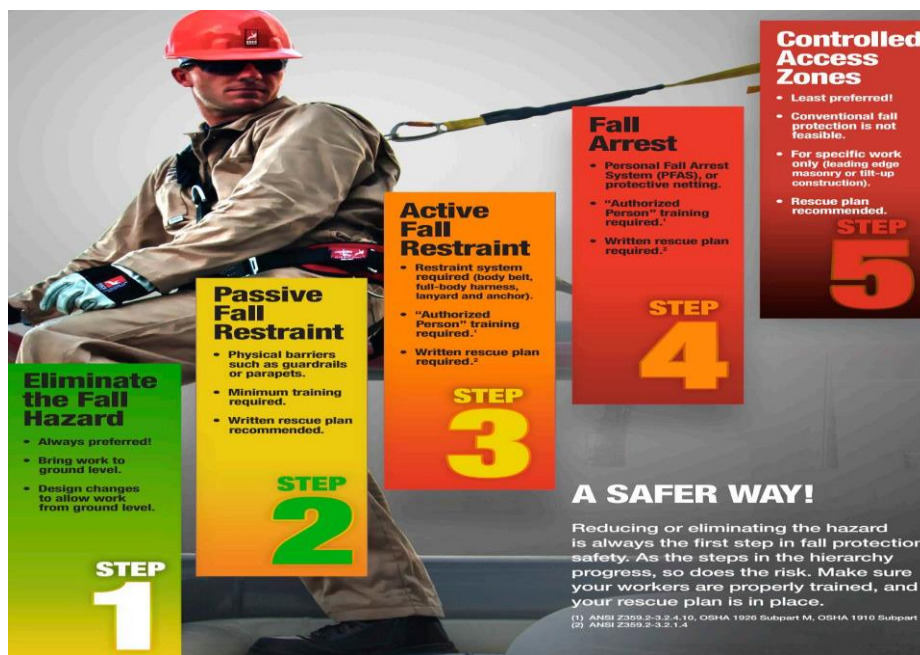
Figure (2.1). Hierarchy of Fall Protection. (Source: Roco Rescue Inc. - Roco Safety Posters, 2017)
